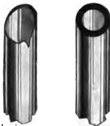
Fig. 5. Erosion or Corrosion of Gage-Glass in Service.
